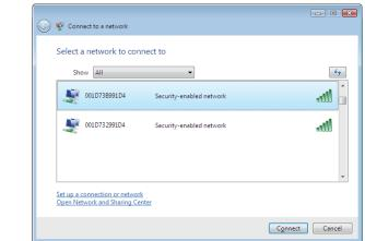
When the screen at left is displayed, select the network to connect to and click [Connect].
