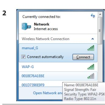
Select the target AirStation's name and click [Connect]. If you will be connecting to this device in the future, checking [Connect automatically] is recommended.
