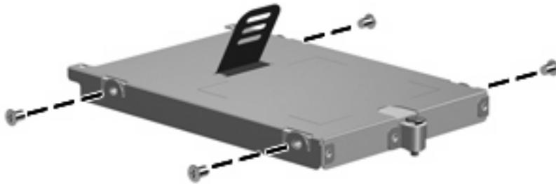
**Where used:** 4 screws that secure the hard drive bracket to the hard drive
