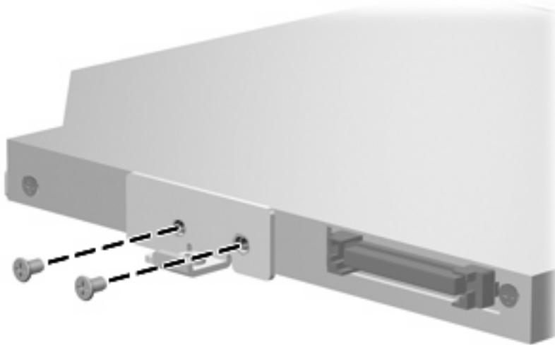
**Where used:** 2 screws that secure the optical drive bracket to the optical drive
