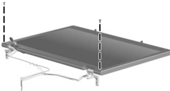
**Where used:** 2 screws that secure the bottom edge of the display bezel to the display assembly
