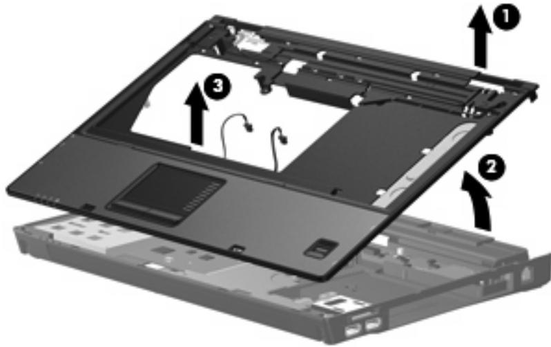
12. If it is necessary to replace the microphone and cable, disconnect the microphone cable (1) from the PC Card/audio board and remove it.
